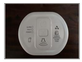
taken. If CO is detected and the alarm sounds, the HUSH button will silence the horn for about 4 minutes. If CO concentrations are above 150 ppm the alarm cannot be silenced.
