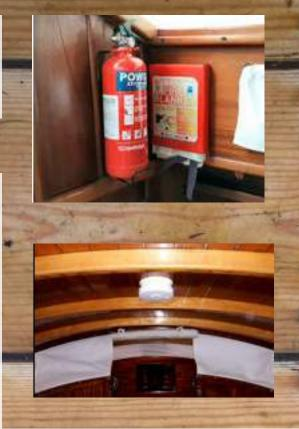
The HUSH control will temporarily desensitise the alarm for approximately 10 minutes when smoke from cooking, etc is expected. The HUSH feature is activated by pressing the test/HUSH button briefly. The LED will then flash every 10 seconds to show that the alarm is in the HUSH mode. The alarm will automatically reset after about 10 minutes but the feature can be used repeatedly. To end the HUSH period, press the test/HUSH button briefly.
