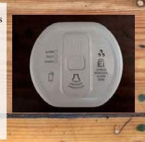
The alarm will bleep and the orange light will flash to indicate a fault. The alarm may sound if aerosols are released nearby.
